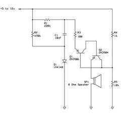
This circuit will generate a square wave at about 440 Hz, depending on the power supply voltage. You could use it as a code practice oscillator by keying the supply voltage. Q1 and Q2 are impersonating a programmable unijunction transistor, which is no longer an easy part to find. This page: <u>Collection of Programmable</u> <u>UJT Circuits</u> has a bunch of interesting circuits you can play with. Get out your breadboard and try a few.
